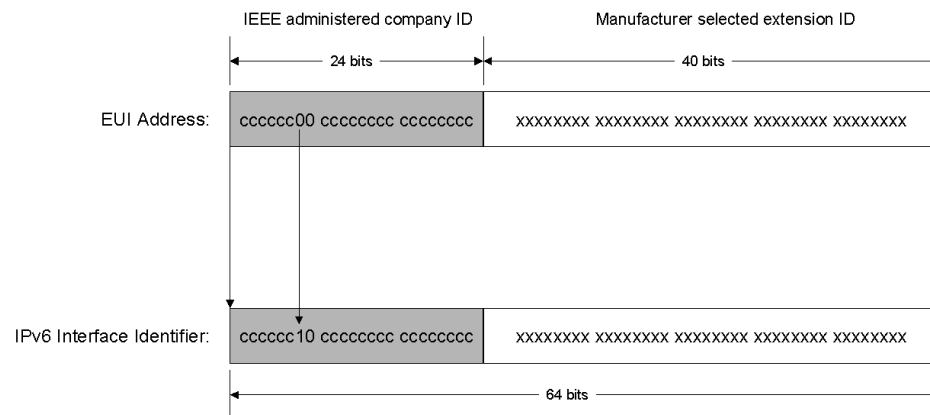
Figure 15 The conversion of a universally administered, unicast EUI-64 address to an IPv6 interface identifier
